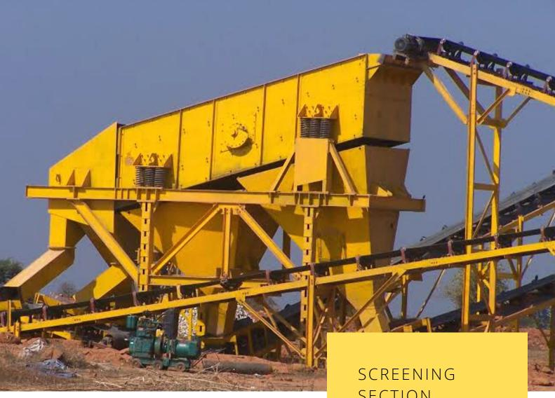
BPA INCLINED SCREENS OFFER RELIABLE AND VERSATILE SCREENING IN AGGREGATES PRODUCTION PLANTS, QUARRIES, GRAVEL PITS AND MINING OPERATIONS. THEIR CIRCULAR MOTION AND VARIABLE SLOPE HELP YOU ACHIEVE A HIGH PRODUCTION CAPACITY AND IMPROVE PROFITABILITY.
